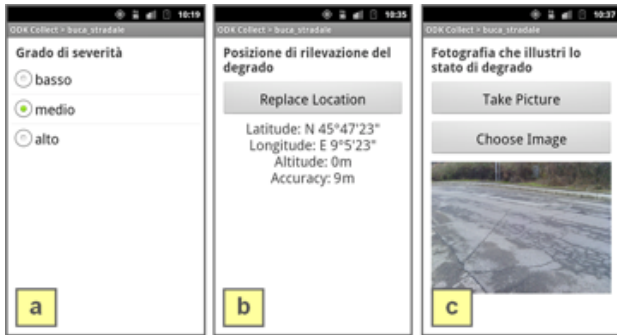
Figure 2: Screenshots of the Android ODK Collect application for reporting pavement damages, showing (a) the choice of the event severity degree, (b) the event position registration using GPS, (c) the event picture taken with the device camera.
